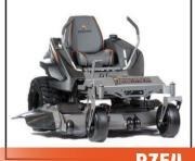
25 HP Briggs Engine, 54" Fabricated Deck,
