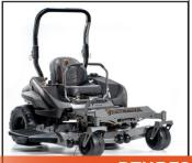
27 HP Kawasaki Engine, 7 Gauge 72" Fabricated Deck, Rear Radial Tires, Suspension Seat, 360 Plate
